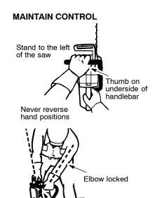
Keep a good, firm grip on the saw with both hands when the engine is running and don't let go. A firm grip will help you reduce kickback and maintain control of the saw. Keep the fingers of your left hand encircling and your left thumb under the front handlebar. Keep your right hand com-pletely around the rear handle whether your are right handed or left handed. Keep your left arm straight with the elbow
